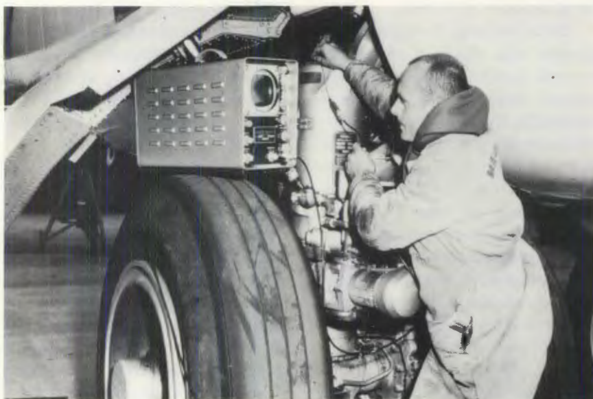
Technician tests main landing gear outer cylinder on a B-52
